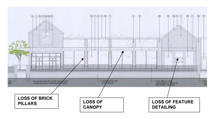
Notable changes from approved elevation to proposed elevation
